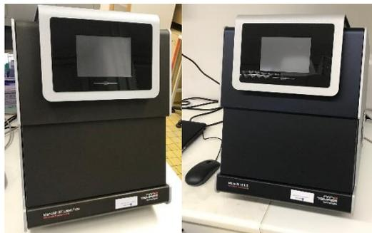
**Prometheus NT.48** device was installed in our laboratory, which utilizes the technique based on the nano differential scanning fluorimetry (nanoDSF) in analysing states and stability of proteins. This device complements the interaction studies as the correct folding and the aggregation state of proteins should be determined before analyses. NanoDSF monitors the fluorescence change of the tyrosine/tryptophan in the structure of the proteins during thermal unfolding.
